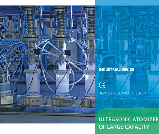
PRIZnano is a large capacity ultrasonic atomizer of liquids. Usage of 3 piezo-electric crystals guarantee a large atomization capacity up to 1.2 l/h, which provides production of large quantity of aerosol that is ideal for independent use (humidification of large spaces) or in combination with other system for the production of nano particles.
